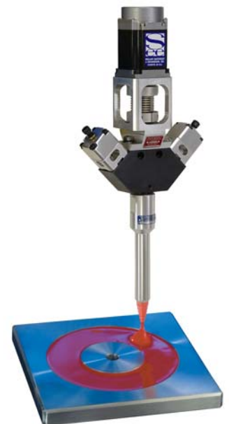
Power Static Mixer Dispensing into a Mold
