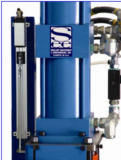
Program-A-Shot Control Option provides Multiple Shot Size Selections
