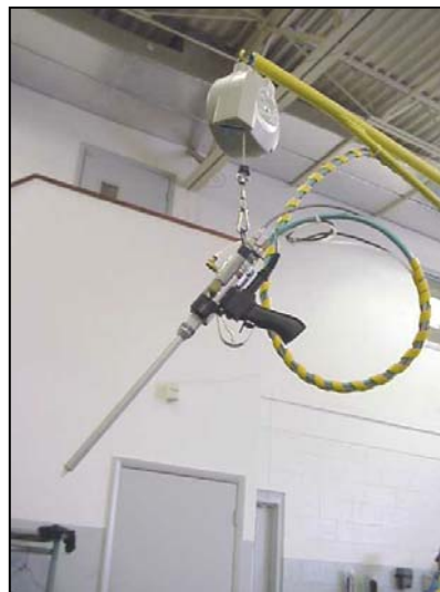
Manual Dispense Valve with No-Flush mixer
