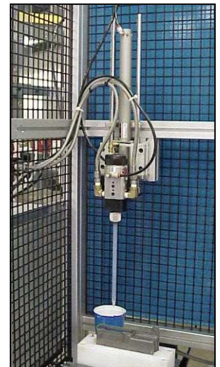
Automatic Dispense Valve on XYZ automation system
