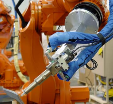
2-Part Valve EOA Tooling with Temperature Controlled Hoses
