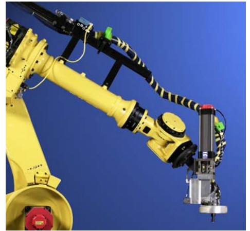
EOA Meter Tooling and Dress-Out
